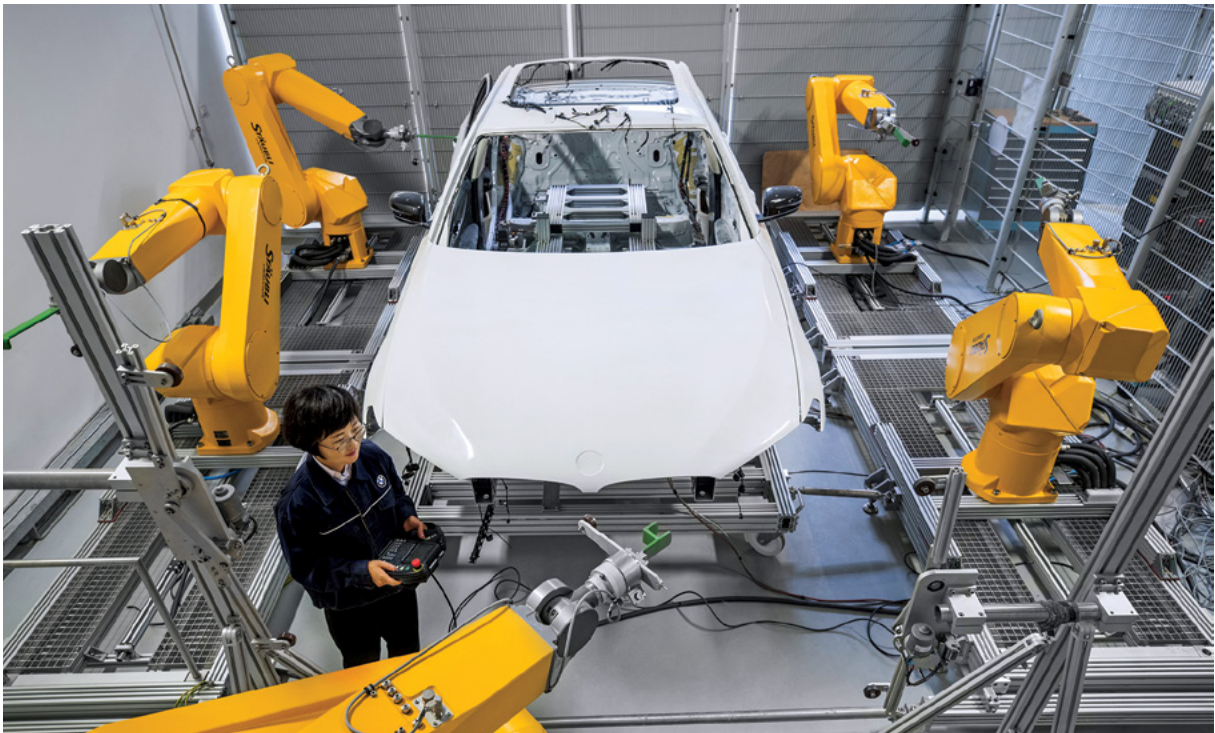
Car doors and flaps test bench in our R & D.
