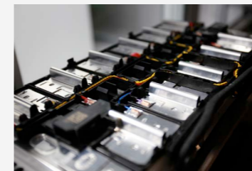
High-Voltage Battery modules are assembled at BMW Brilliance HVB Centre.
